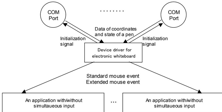
Fig. 2. Data and control flow of the device driver.
