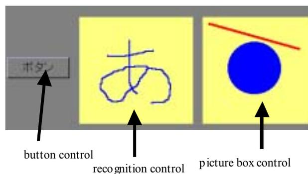
Fig. 3. The controls for simultaneous inputs with multiple electronic pens.
