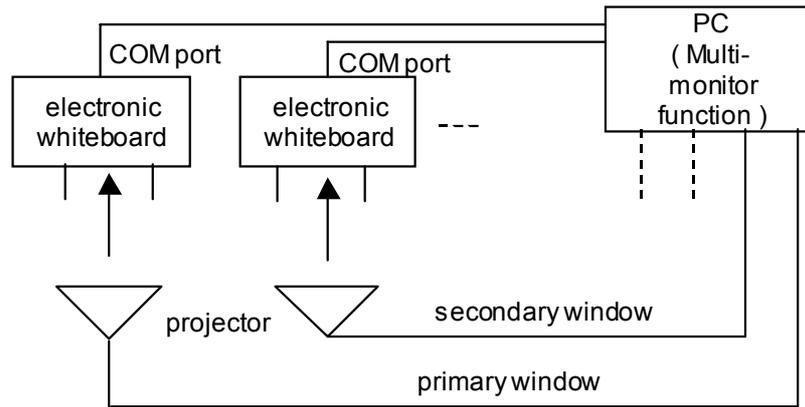
Fig. 1. Hardware configuration (employing the front projection type).
